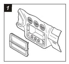
Disconnect the negative battery terminal to prevent an accidental short circuit. Unclip the radio trim bezel. Remove (4) 7mm hexhead screws securing the factory head unit and disconnect the wiring.
